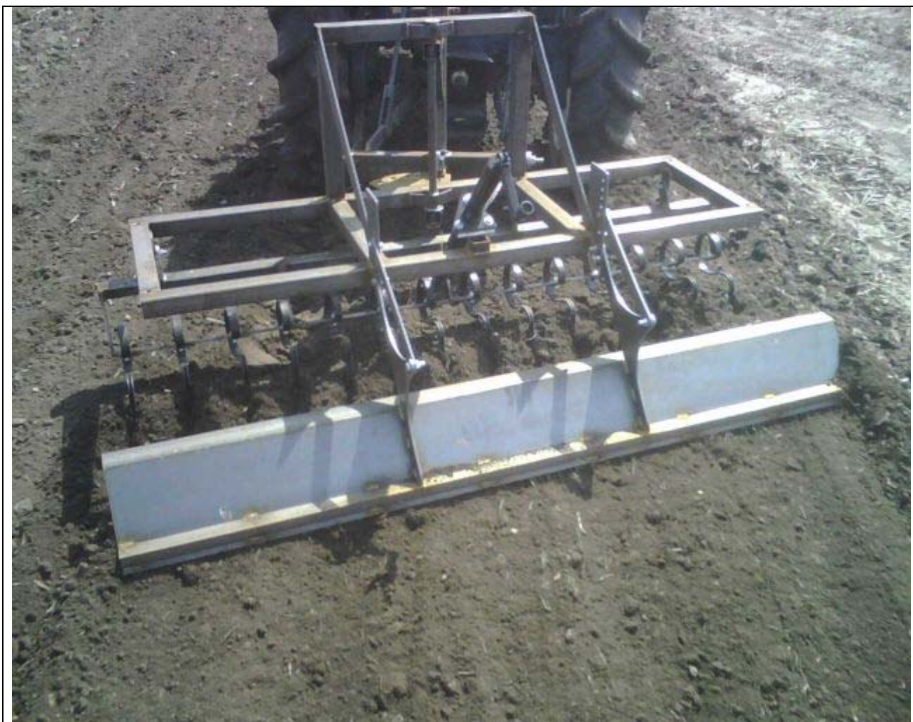
TAG 7 Grooming with the Blade at 30 degrees
