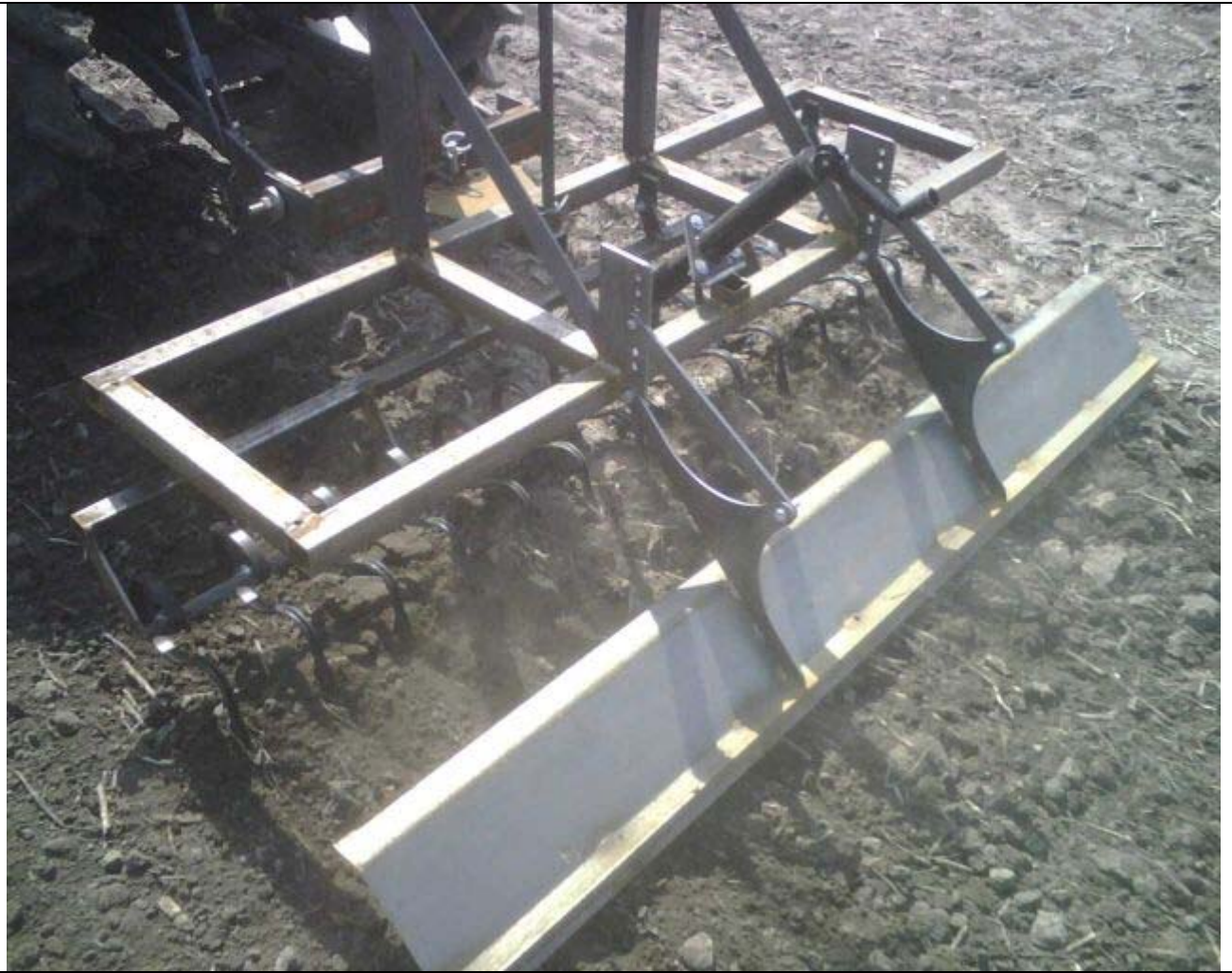
TAG 7 Grooming with the Blade at 0 degrees
