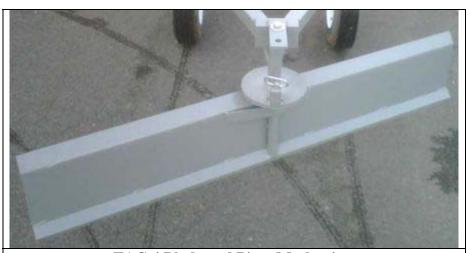
**TAG 4 Blade and Pivot Mechanism**
